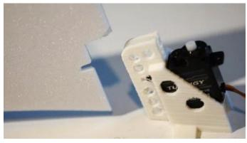
Glue a CFK rod into the rudder adaper.
