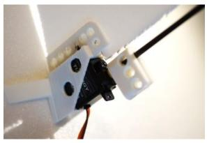
On the upper edge of this Depron part, glue the **rudder backup**. Make sure the 3 mm hole is vertically above the servo horn.
