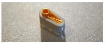
If the snap fit of the servo in the **servo adapter** is not rugged, glue the servo into the **rudder adapter**. Or use just tape, to remove the servo later.
