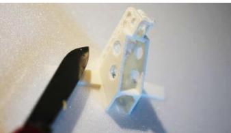
3x **Rudder backup**: Use a knife to clean the part from printing remains in a way that the depron fits in the lower part and a thin cord goes easily through the two holes. Use a 3 mm drill to open the big hole.
