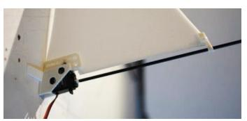
Glue the rudder part of the Depron into the **rudder adapter** and to the **13 cm CFK rod**. Shape the moveable rudder part as you wish, that's the individual part of your silent runner and we love to see different shapes. Slow indoor ships should have big rudders (18 cm long) faster ships use shorter rudders.
