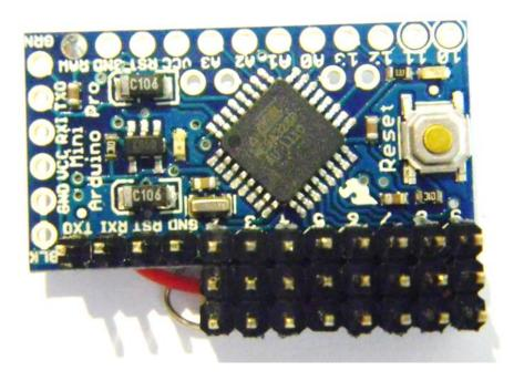
The final Arduino looks like this. Note that all the pins on the top are free to use and provide amazing capabilities for advanced functions. Servo cable will be connected with the SIGNAL (white/orange) to the Arduino pins, the middle pin to +5V RED and the lower pin to GND BLACK
